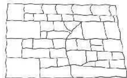
Random rubble masonry
